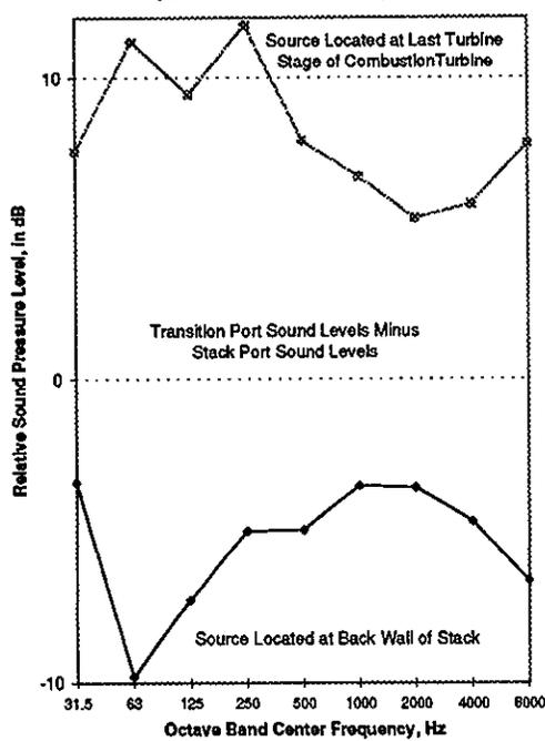
Figure 8. Relative Sound Levels Measured at the Exhaust Transition Probe and at the Probe Located in the Back of the Stack with the Combustion Turbine Operating
