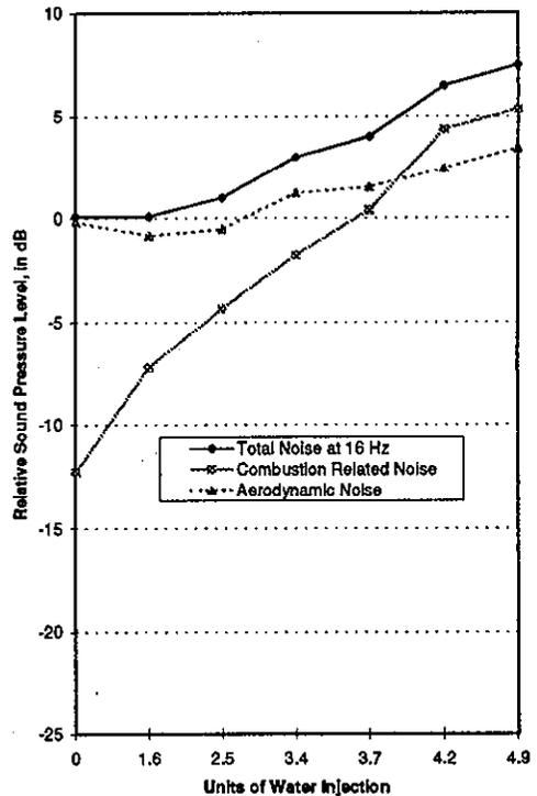
Figure 5. Relative Sound Level Contribution of Combustion and Aerodynamic Sources at 31.5 Hz Based on Coherent Output Power Estimates
