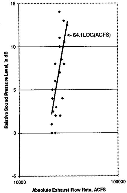
Figure 7. Effect of Source Location on Measured Sound Level (ILG Source with Cold Stack)
