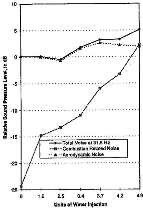
Figure 6. Changes in Sound Pressure in the 31.5 Hz Octave Band with Exhaust Flow
