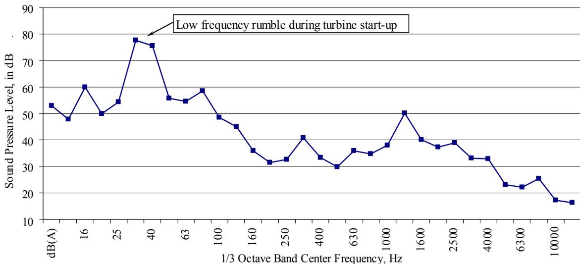
Figure 2: Low frequency rumble of combustion turbine at startup.
