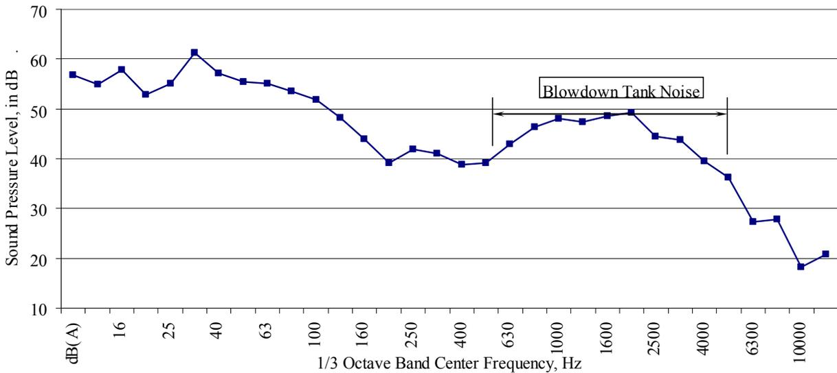
**Figure 4:** Blowdown tank noise measured within the community without a silencer.
