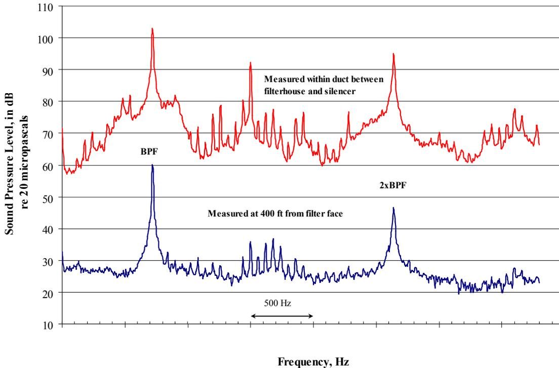
**Figure 1:** Tonal noise from a problematic gas-turbine air-inlet silencer.
